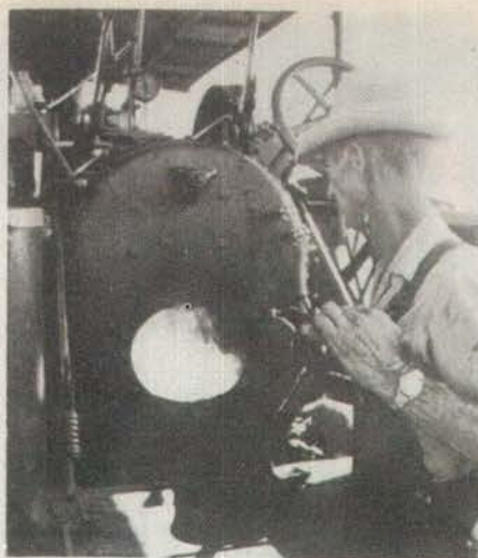
Ewell Hollingsworth, who harvested his 1965 wheat crop with the thresher, checks the steam boiler which will burn either wood or coal.
