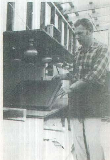
Thomas Travis holds a fiberglass mold for a square cultured marble table top. This mold is treated to give the marble a slick polished finish. The heat lamps aid the curing process.
