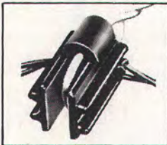
RP-12 — ROUND POST INSULATOR — String the wire — slip it on and plastic nut locks insulator in place. Simple — sturdy — nothing to rust. For 3/8" post. RP-13 — 1/2" post.
