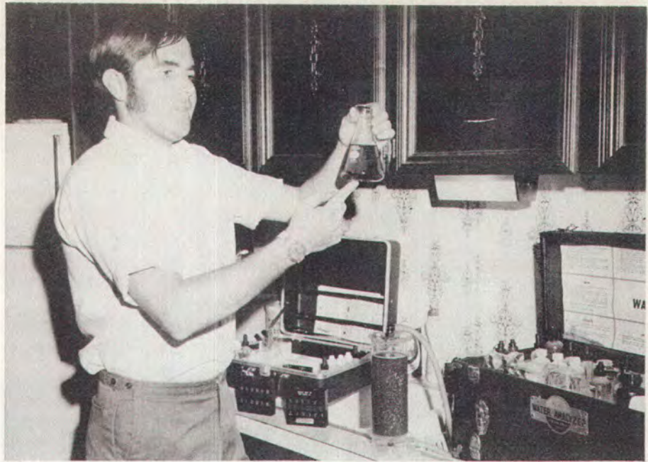
Johnny Chambers (above) owner and operator of Chambers Water Purification Equipment, Inc. is shown making a water test to determine the specific pieces of equipment needed to obtain pure water at the customer's home.
