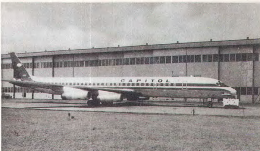
This Capitol International Airways DC-8 jet will carry 250 passengers at up to 600-miles-per-hour comfort. It has a non-stop capability of 5,000 miles and carries a crew of eleven.
